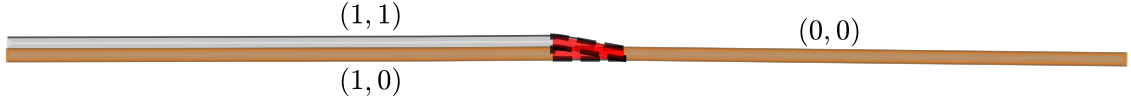
Figure 2.2.: Lane Network for example 1. Brown shows start- and end lanes for both vehicles. The critical section between intersecting lanes is given in red (more in Section 3.2.1).
